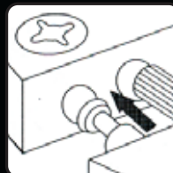
3. Join panels, inserting studs and dowels into the corresponding holes.
