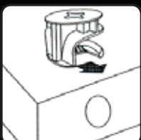
1. Place cam locks in pre drilled holes.
