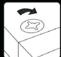
4. Tighten cam locks in a clockwise direction.
