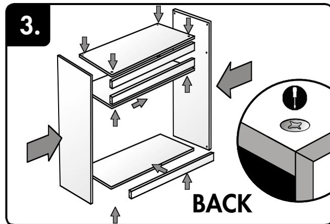
Connect side panels to all 3 support rails and top, mid horizontal shelf and cupboard bottom, then fasten cam locks.
