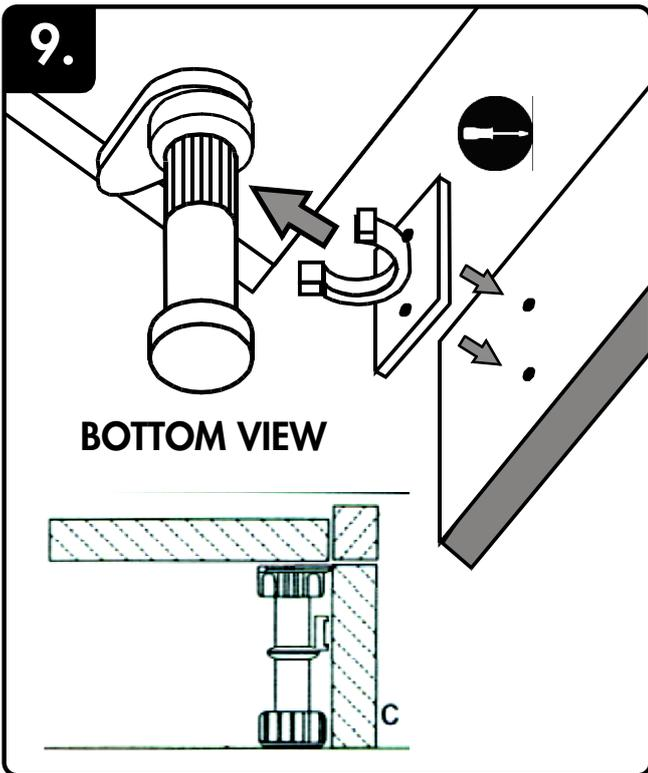
Each leg has a plate on it with a semi-circular clip attached which clips on to the shaft of the leg. Screw the plates onto the corresponding positions on the skirting first and then clip the entire skirting onto the legs.
