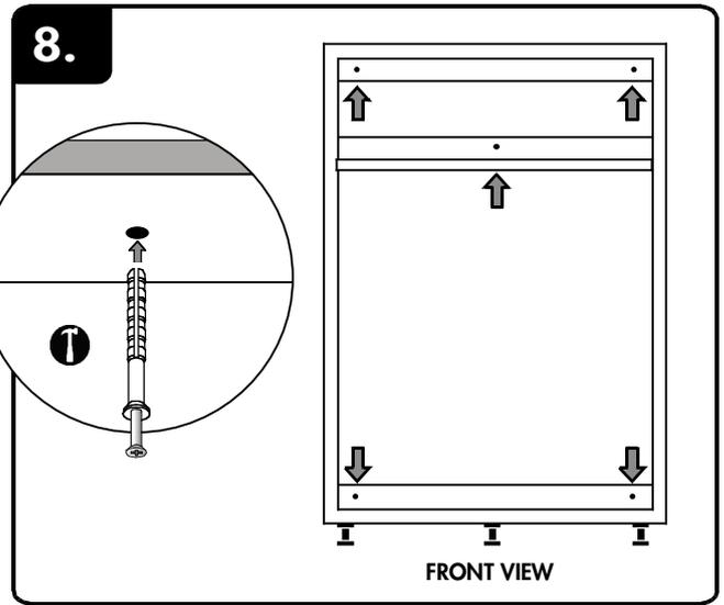
Place the cupboard in its final position and drill 5 holes for wall plugs – 2 go through the top rail into the wall, 2 in the bottom rail and the last one centered in the middle rail. Insert the wall plug into the holes, and hammer into place.
