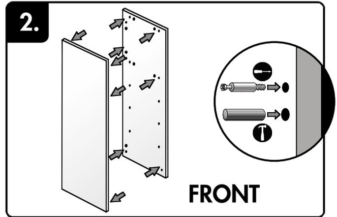
Screw studs and gently knock dowels into pre-drilled holes in side panels. The unit must be assembled on a firm smooth surface as to avoid damaging the panels. Dowels may also puncture the back of the panel if there is no resistance on a soft surface.
