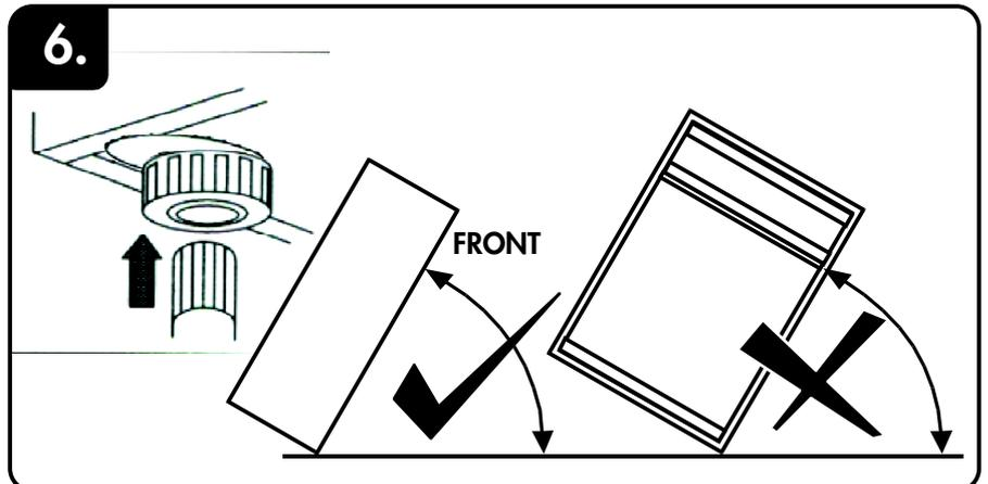
Insert the rest of the leg into the base section. This will be done as the unit is maneuvered into position. Care must be taken to use only the front or back leading edge – not the side edges – when raising the unit into position, or it may be damaged.
