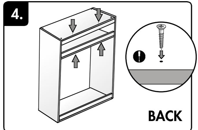
Screw support rails into top, mid horizontal shelf and cupboard bottom.
