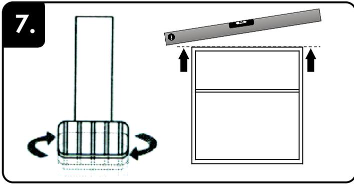
Adjust the other ends of all 6 of the legs until the unit sits level and stable on the ground. Always use a spirit level to ensure cupboard is level when fixing it to the wall. If unit is not level the installation will not be successful.
