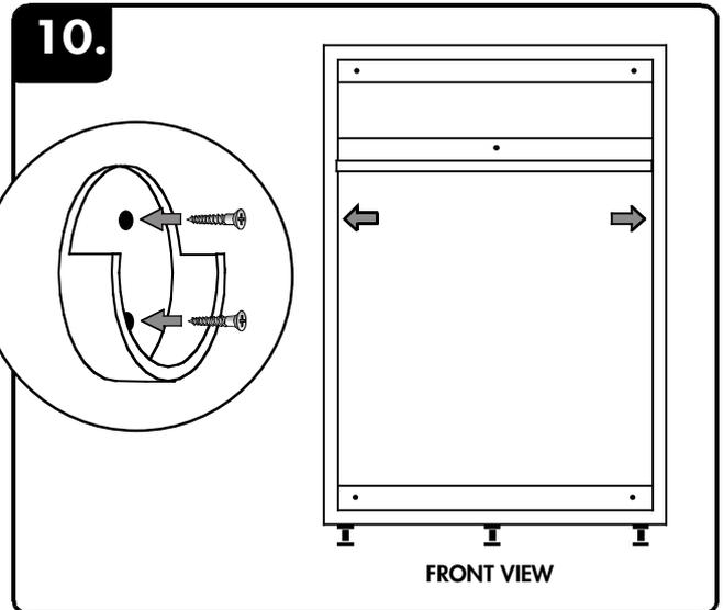
Attach the two hanging rail flanges to the inside of the cupboard as shown, taking care to centre them between the front and back of the cupboard.
