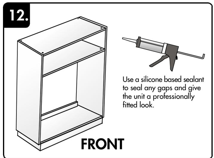
Use a silicone based sealant to seal any gaps and give the unit a professionally fitted look.
