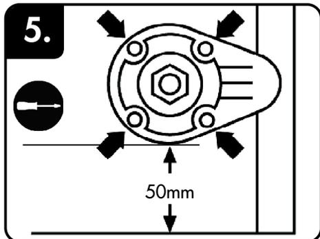
Mark lines along the base 50mm from the front and back of the unit. Line up the base section of the foot with this line and screw in, ensuring the flange goes over the join with the side panel for added stability. Note that the placement of the base overlapping the side panel does not apply for an exposed side, as it will interfere with the skirting board.
