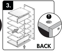
Join side panel and support rails then fasten cam locks.
