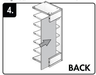
Insert back panel into groove in top and side panels.
