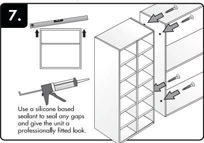
Place the cupboard in its final position and screw the unit into position from the adjacent unit, so that they attach flush to each other. Always use a spirit level to ensure unit is level when fixing it to the adjacent unit.
