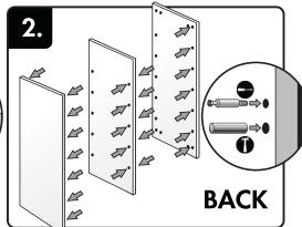
Screw studs and press dowels into pre-drilled holes in side panels and both sides of centre divide.
