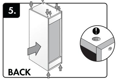
Join second side and fasten cam locks into position. Screw back rails into position.
