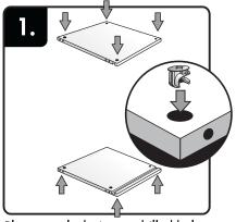
Place cam locks in pre drilled holes, in top and bottom panel with grooves facing inward.
