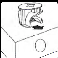
1. Place cam locks in pre drilled holes.
