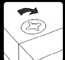
4. Tighten cam locks in a clockwise direction.
