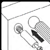
2. Screw studs and press dowels into pre drilled holes in side panels.
