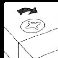
4. Tighten cam locks in a clockwise direction.
